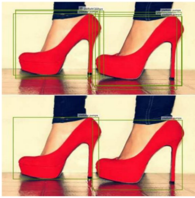
Figure 3: Non Maximum Suppression applied to the detection results
